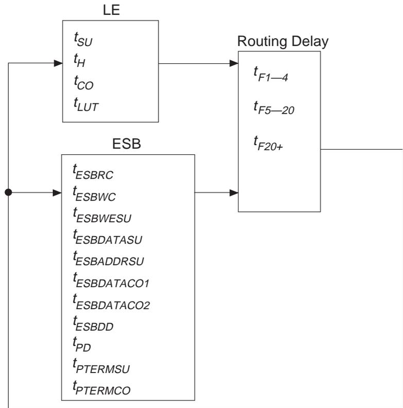
Figure 37 shows the  $f_{MAX}$  timing model for APEX 20KE devices. These parameters can be used to estimate  $f_{MAX}$  for multiple levels of logic. Quartus II software timing analysis should be used for more accurate timing information.
