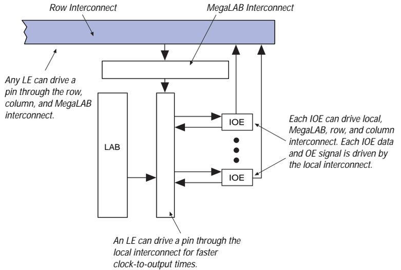
Figure 28 shows how a column IOE connects to the interconnect.
