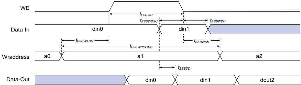
Figure 39. ESB Synchronous Timing Waveforms
