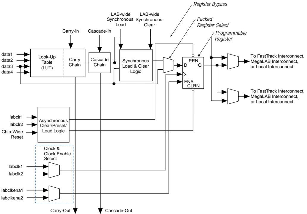
Each LE's programmable register can be configured for D, T, JK, or SR operation. The register's clock and clear control signals can be driven by global signals, general-purpose I/O pins, or any internal logic. For combinational functions, the register is bypassed and the output of the LUT drives the outputs of the LE.
