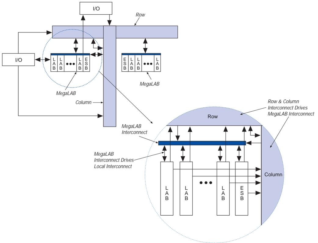
Figure 11 shows the intersection of a row and column interconnect, and how these forms of interconnects and LEs drive each other.
