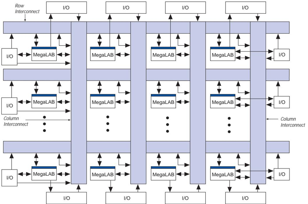
A row line can be driven directly by LEs, IOEs, or ESBs in that row. Further, a column line can drive a row line, allowing an LE, IOE, or ESB to drive elements in a different row via the column and row interconnect. The row interconnect drives the MegaLAB interconnect to drive LEs, IOEs, or ESBs in a particular MegaLAB structure.
