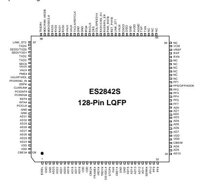
Figure 1 ES2842 Pinout Diagram
