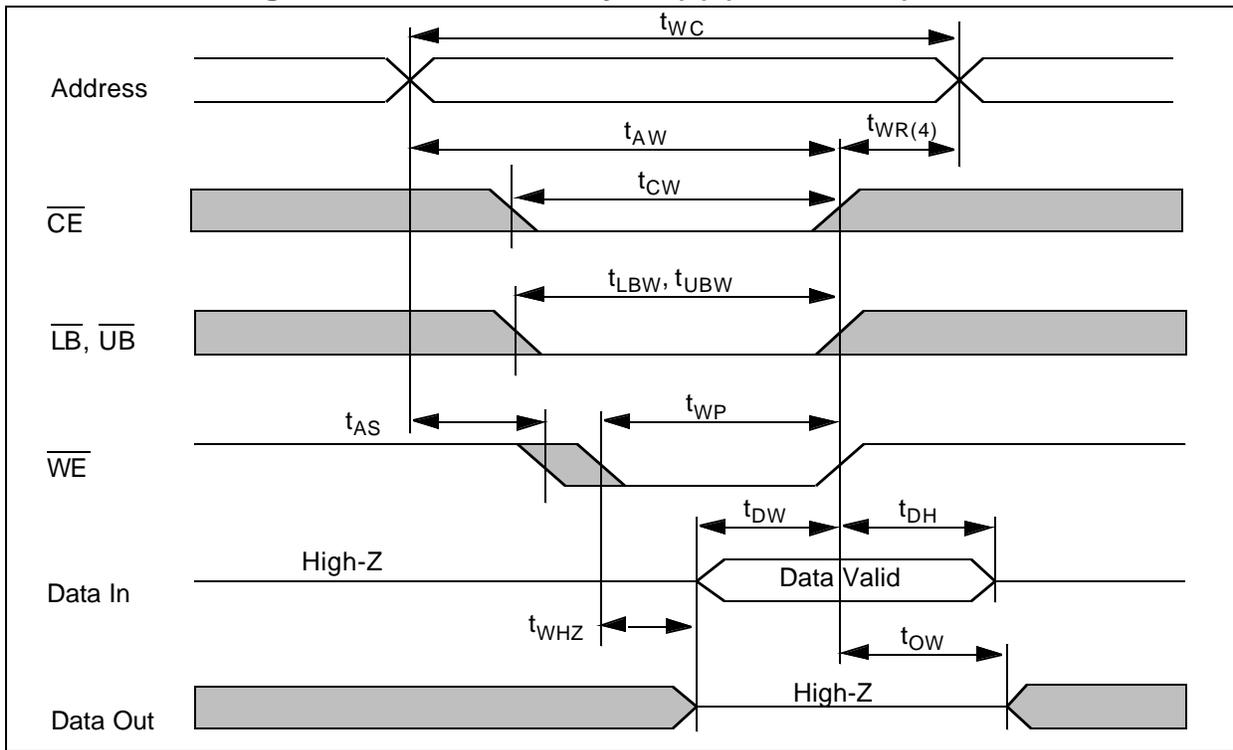
**FIGURE 7: Timing Waveform of Write Cycle (2) ( $\overline{CE}$  Control)**
