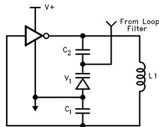
$C_1$  is to adjust the center frequency,  $C_2$  DC isolates the control from the oscillator, and  $V_1$  is the primary control device.  $C_2$  should be much larger than  $C_V$  so that  $V_1$  has maximum modulation capability. The frequency of oscillation is given by:
