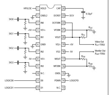
Note: Pin #6 should be a good high frequency ground
