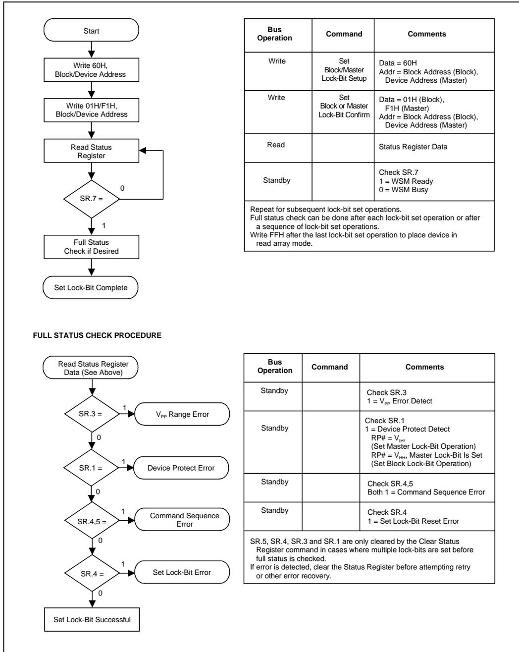
Figure 10. Set Block and Master Lock-Bit Flowchart
