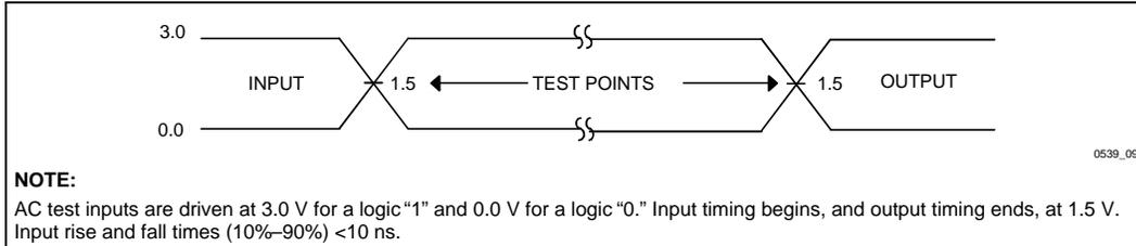
Figure 17. 3.3 V Input Range and Measurement Points
