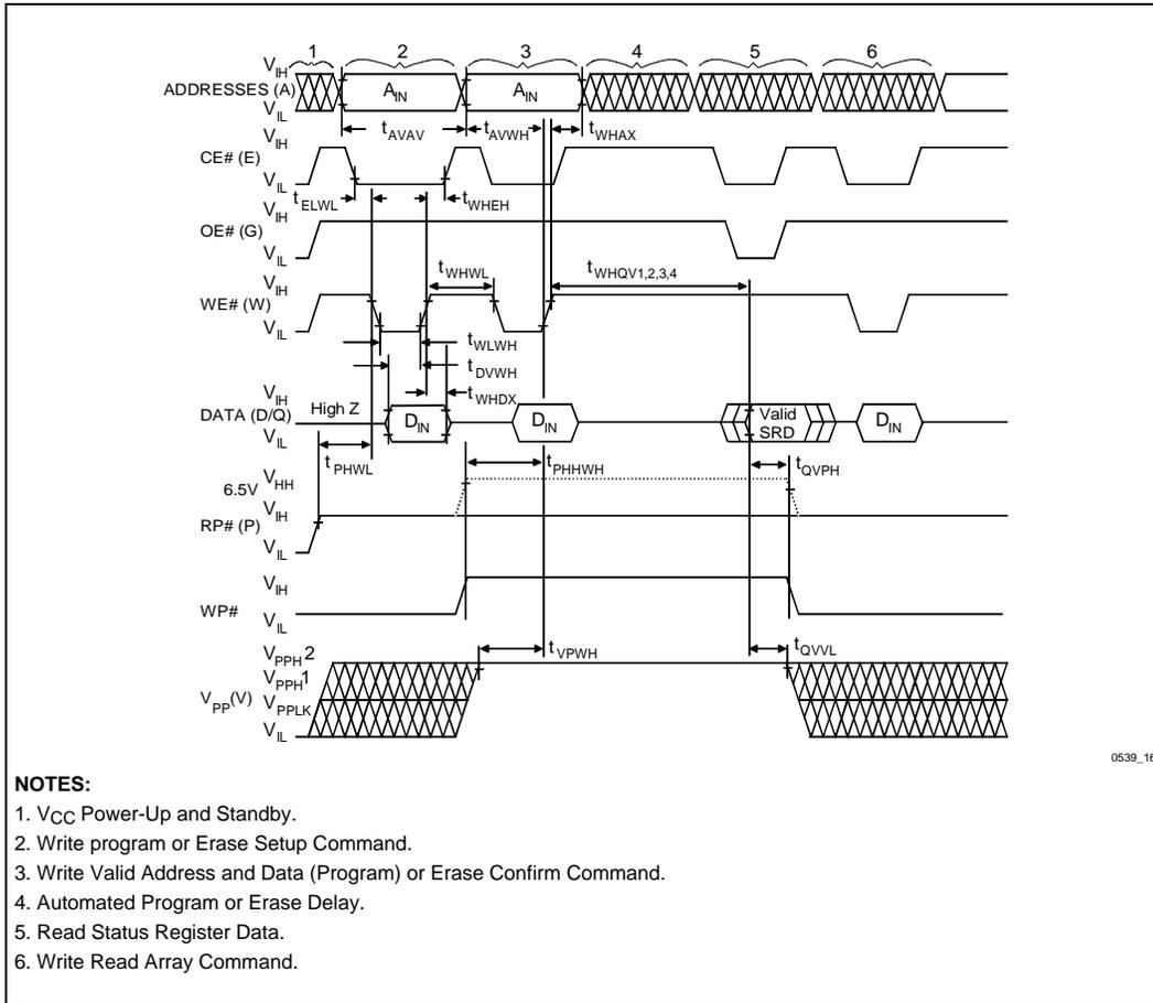
Figure 14. AC Waveforms for Write Operations (WE#-Controlled Writes)
