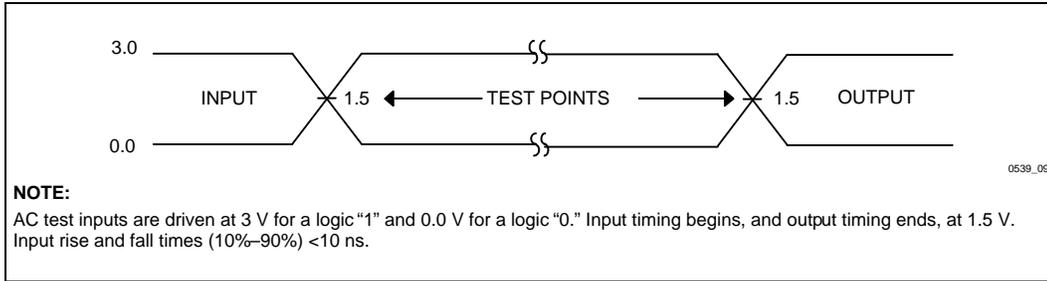
Figure 9. 3.3 V Inputs and Measurement Points
