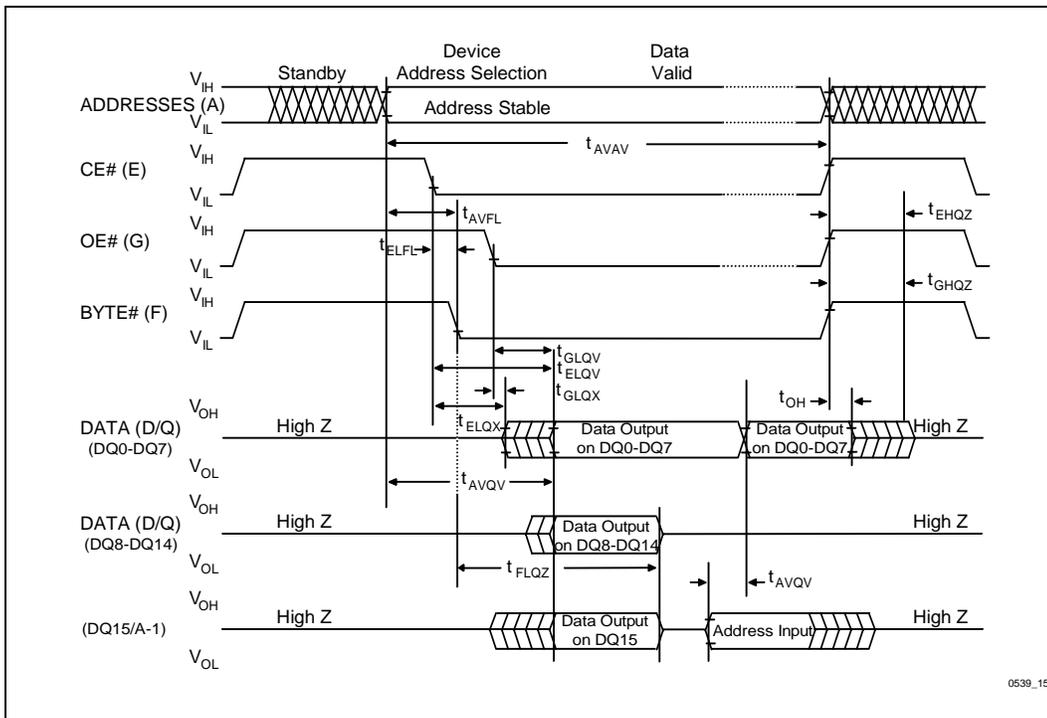
Figure 13. BYTE# Timing Diagram for Read Operations
