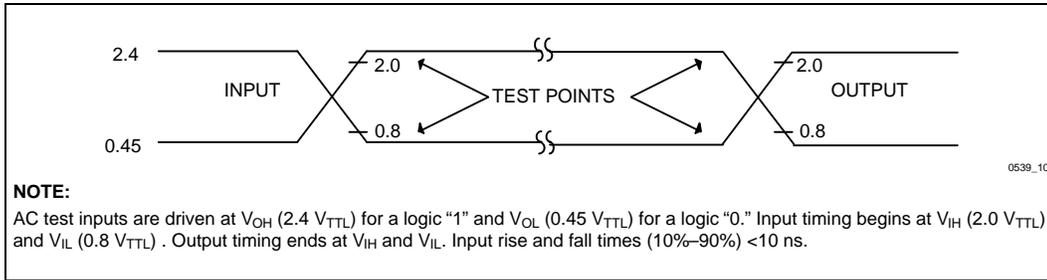
Figure 10. 5 V Inputs and Measurement Points
