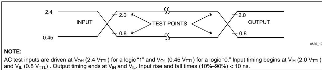
Figure 18. 5 V Input Range and Measurement Points
