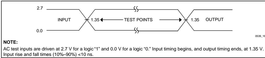
Figure 16. 2.7 V–3.6 V Input Range and Measurement Points
