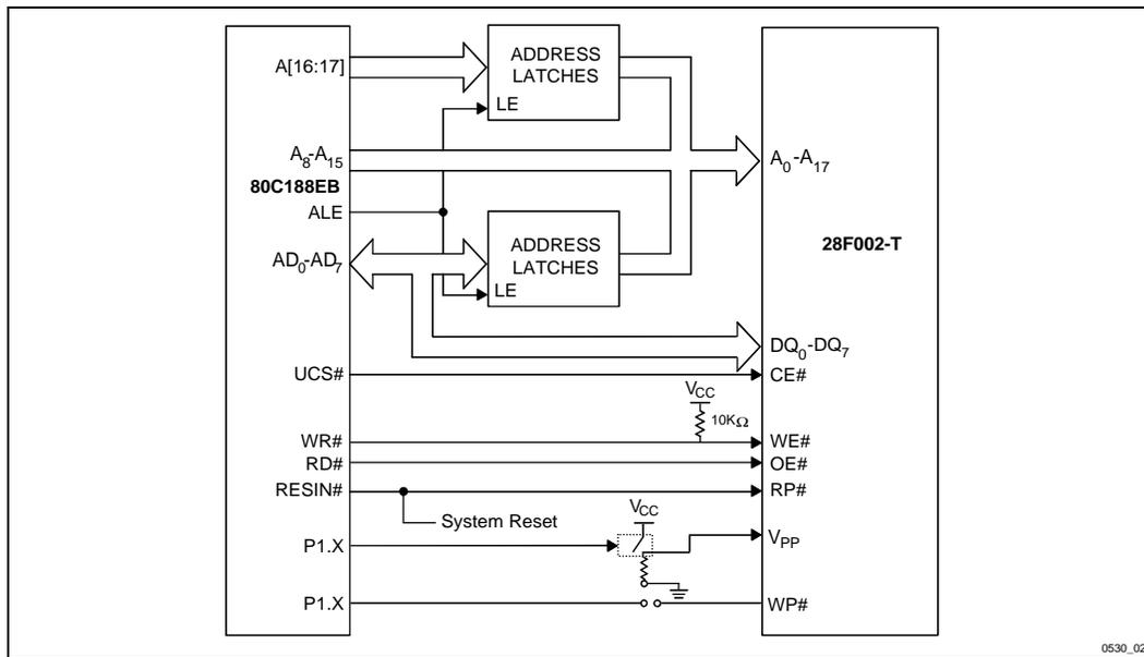
Figure 2. 28F002B Interface to Intel80C188EB 8-Bit Embedded Microprocessor
