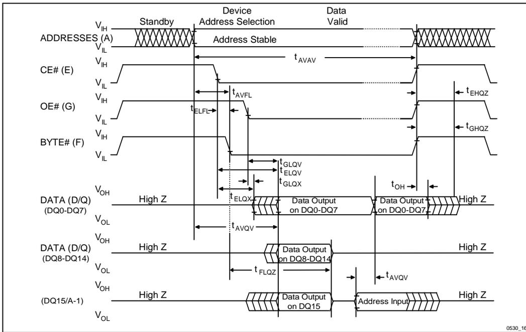
Figure 16. BYTE# Timing Diagram for Read Operations
