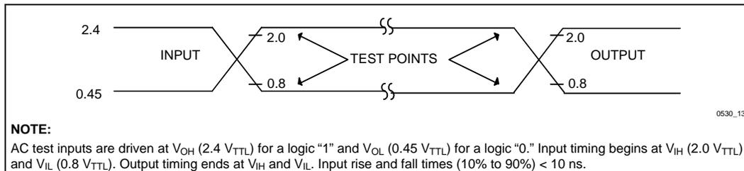
**Figure 20. 5 V Input Range and Measurement Points**
