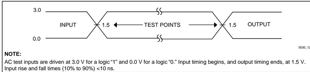
**Figure 19. 3.3 V Input Range and Measurement Points**
