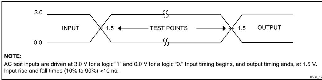
Figure 12. 3.3 V Inputs and Measurement Points
