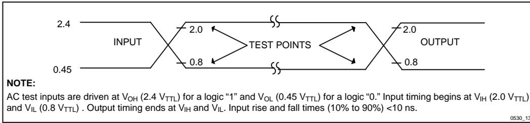
Figure 13. 5 V Inputs and Measurement Points
