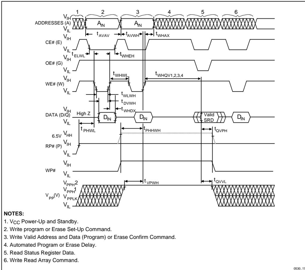
Figure 17. AC Waveforms for Write Operations (WE#-Controlled Writes)
