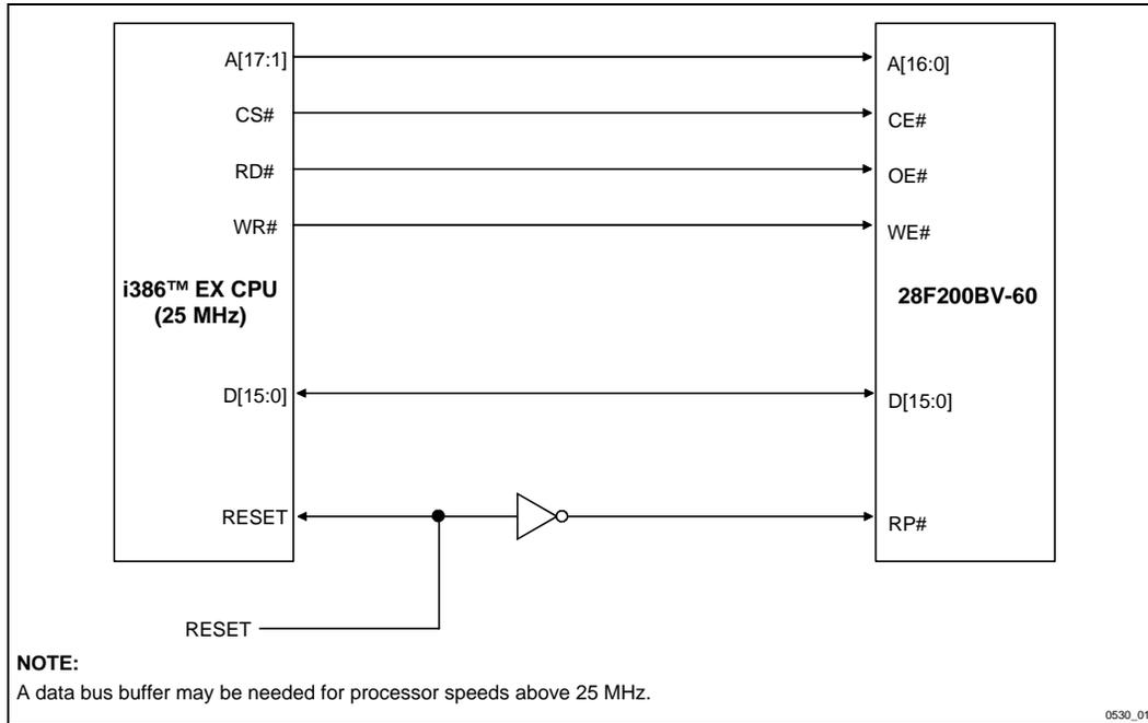
Figure 1. 28F200 Interface to Intel386™ EX Microprocessor
