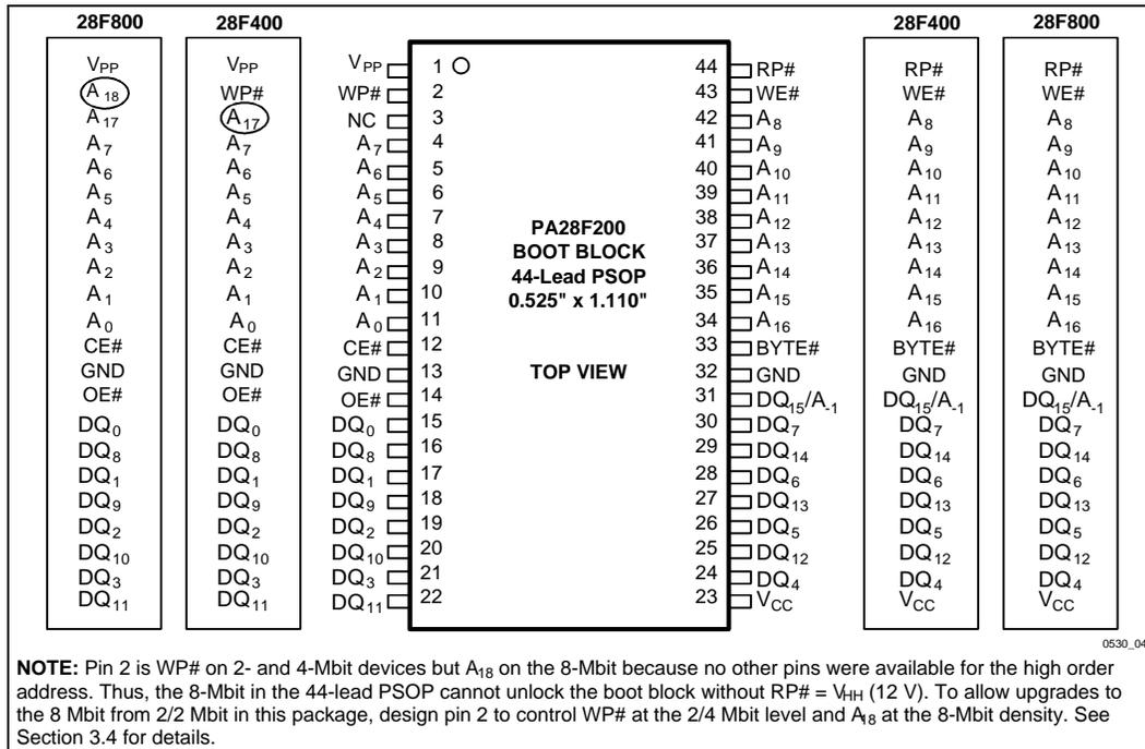
**NOTE:** Pin 2 is WP# on 2- and 4-Mbit devices but A<sub>18</sub> on the 8-Mbit because no other pins were available for the high order address. Thus, the 8-Mbit in the 44-lead PSOP cannot unlock the boot block without RP# = V<sub>HH</sub> (12 V). To allow upgrades to the 8 Mbit from 2/2 Mbit in this package, design pin 2 to control WP# at the 2/4 Mbit level and A<sub>8</sub> at the 8-Mbit density. See Section 3.4 for details.
