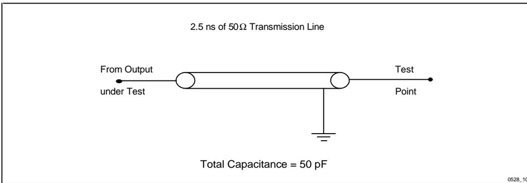
**Figure 10. Transient Equivalent Testing Load Circuit**
