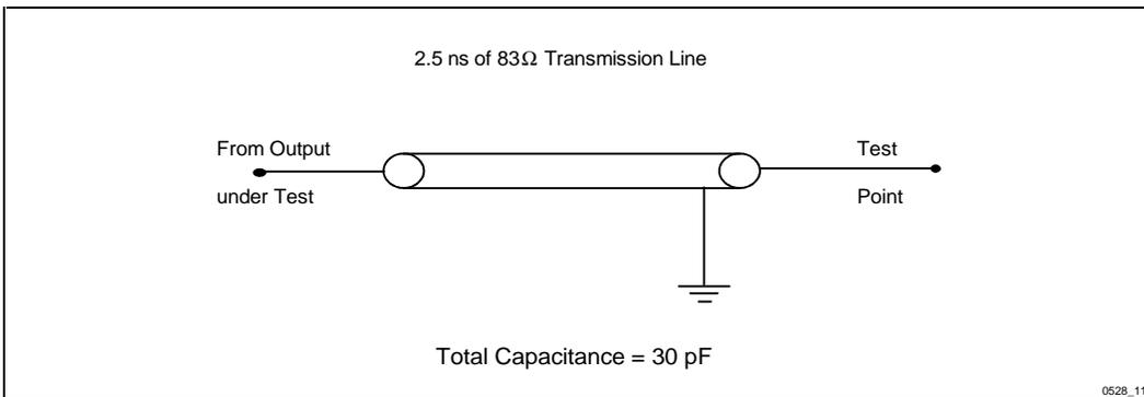
**Figure 11. High Speed Transient Equivalent Testing Load Circuit**
