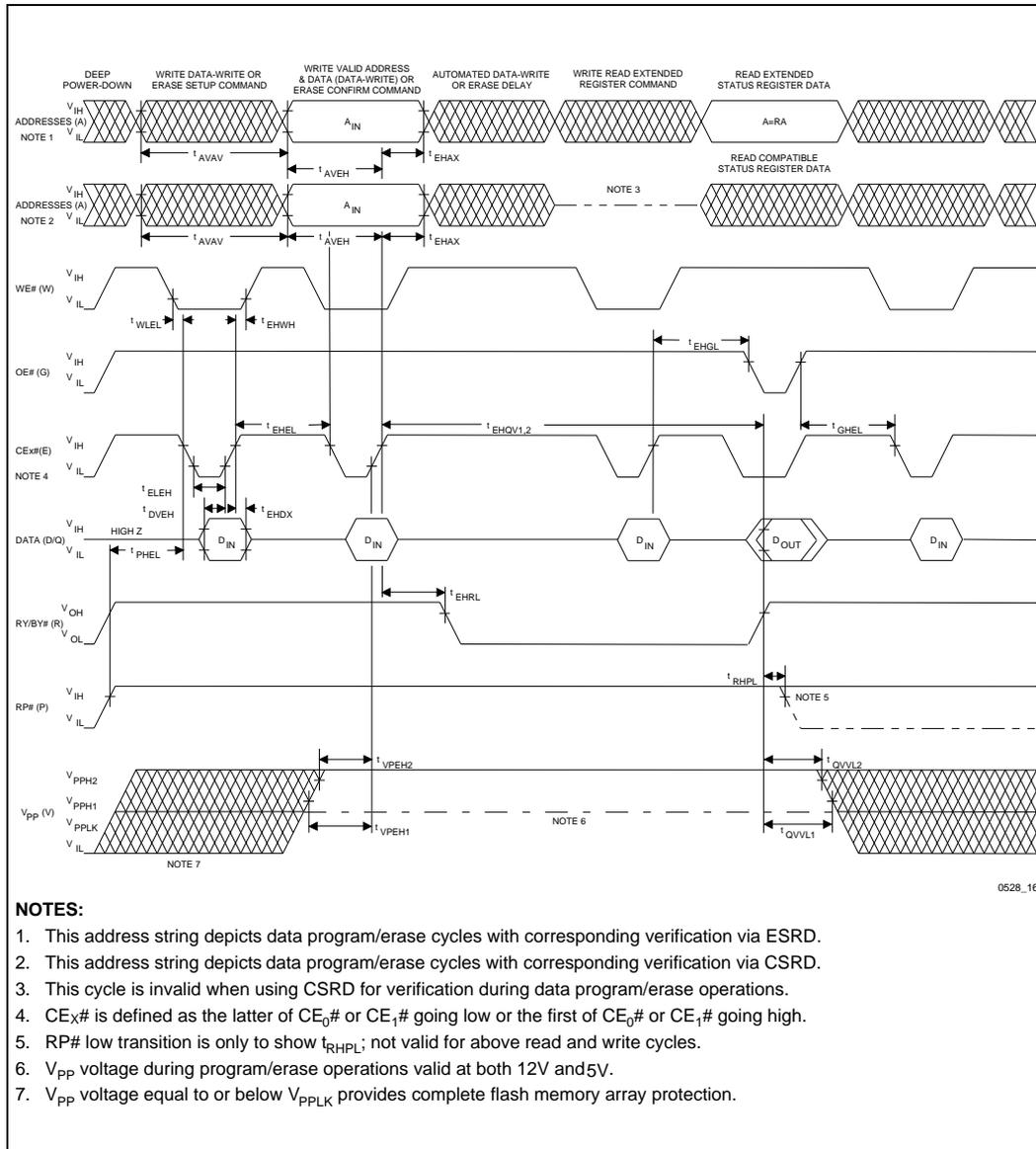
Figure 16. Alternate AC Waveforms for Command Write Operations
