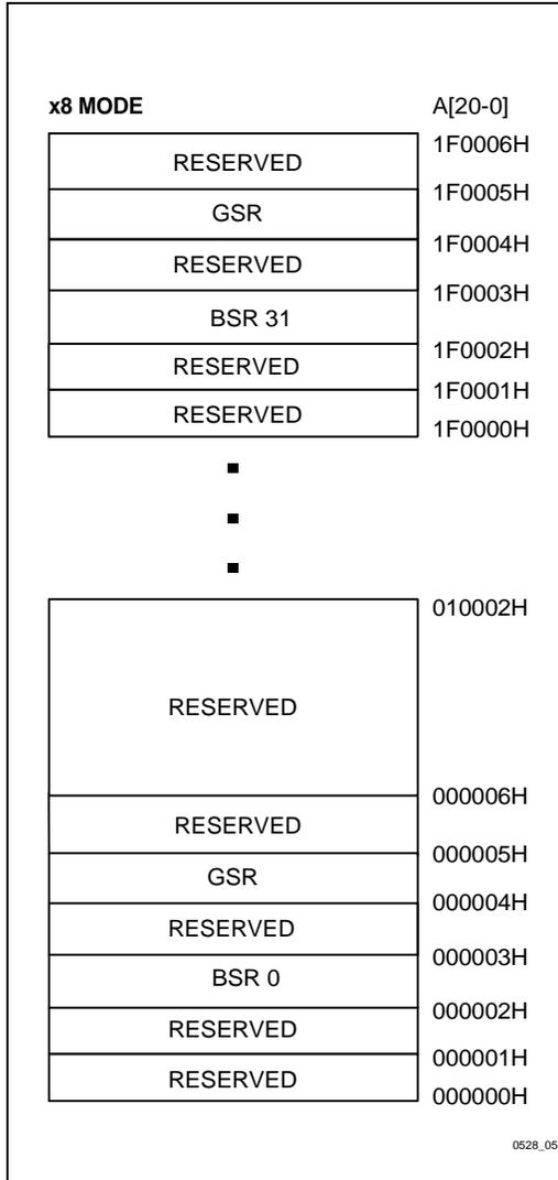
Figure 5. Extended Status Register Memory Map (Byte-Wide Mode)
