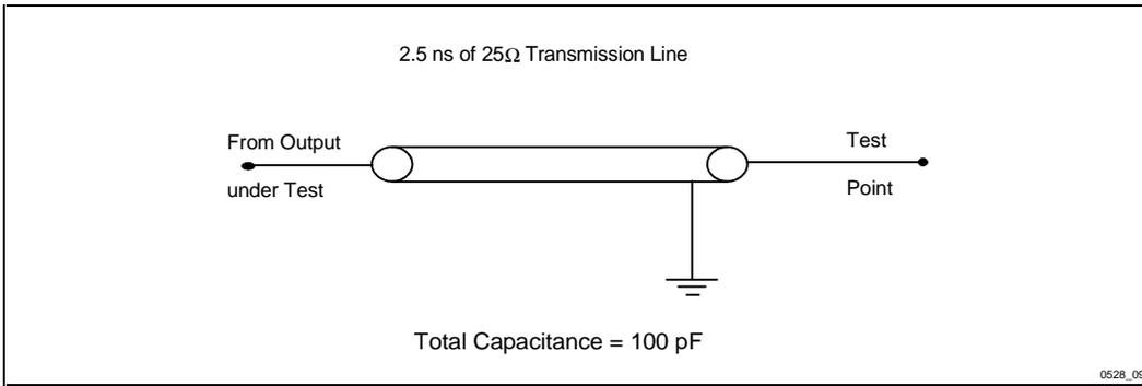
**Figure 9. Transient Equivalent Testing Load Circuit**
