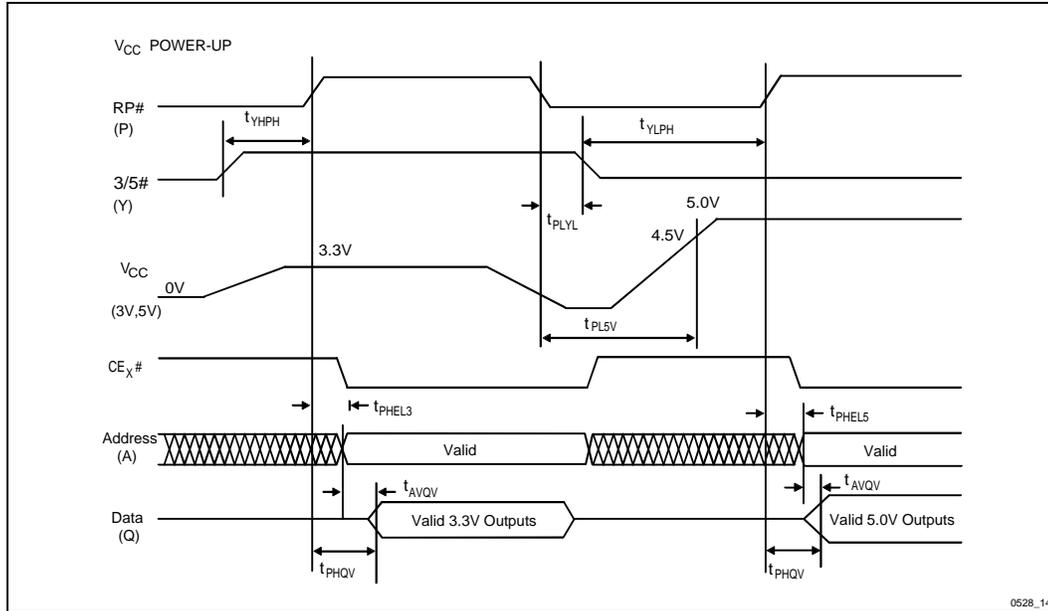
Figure 14. V<sub>CC</sub> Power-Up and RP# Reset Waveforms
