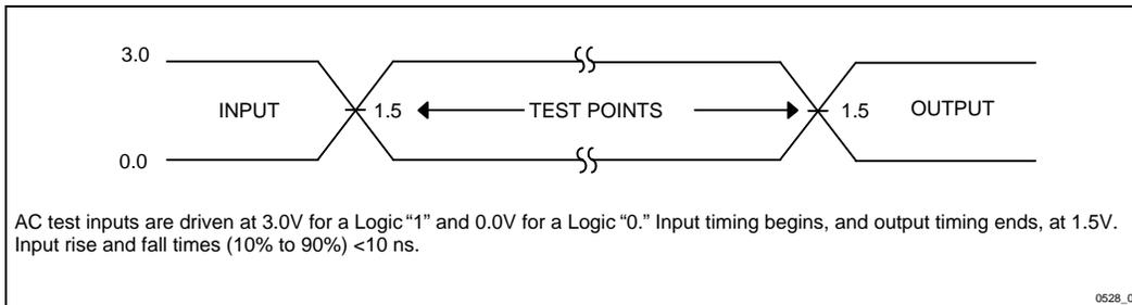
**Figure 8. Transient Input/Output Reference Waveform for  $V_{CC} = 3.3V \pm 0.3V$  and  $V_{CC} = 5V \pm 5\%$  (High Speed Testing Configuration)(<sup>2</sup>)**
