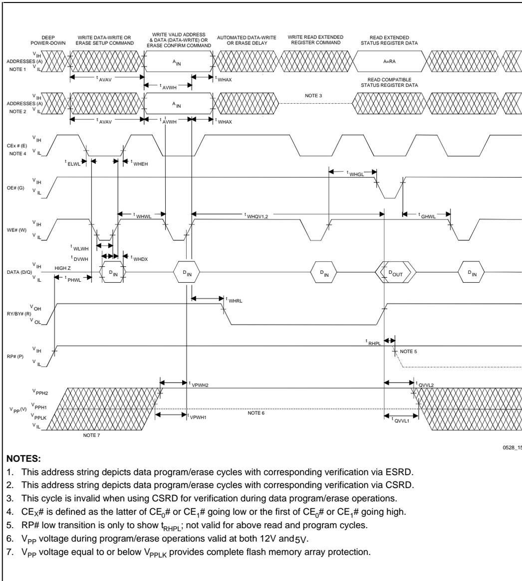
Figure 15. AC Waveforms for Command Write Operations
