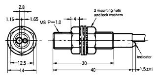
Do not exceed the torque listed in the table below when tightening the mounting nuts.
