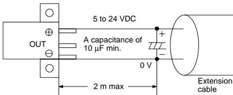
Do not solder the cable to the connectors. Use the EE-1002 Connector or EE-1003 Connector (with a 1-m cable attached) to connect the cable to the output terminals.
