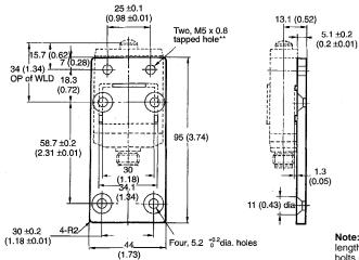
Note: Four hexagonal flat head bolts (M5 x 0.8, length: 10) and two hexagonal head
