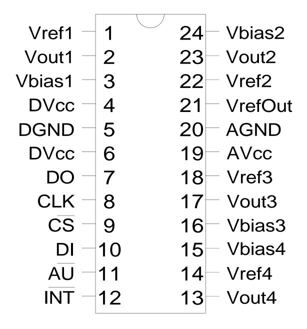
DAC1054CMJ/883 CONNECTION DIAGRAM 24 - LEAD DIP (TOP VIEW) P000003A
