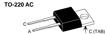
A = Anode, C = Cathode, TAB = Cathode
