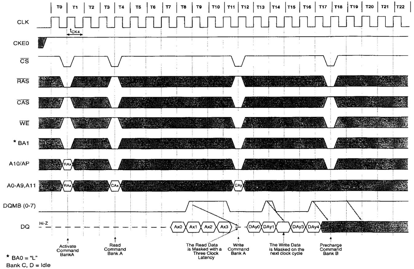
Interleaved Column Read Cycle
