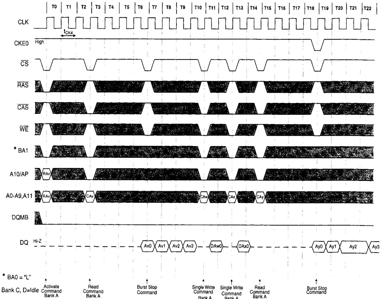
‡ Note that Single Write Operation is possible through programming of the Mode Register.
