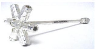
Microlab/FXR Model D2-D6 Power Splitters have been designed to evenly split high power signals with minimal reflections or loss. Units may also be used as low loss coherent combiners provided all inputs are both amplitude and phase coincident. Designed with only a few solder joints and an air dielectric, the loss has been minimized and reliability enhanced.
