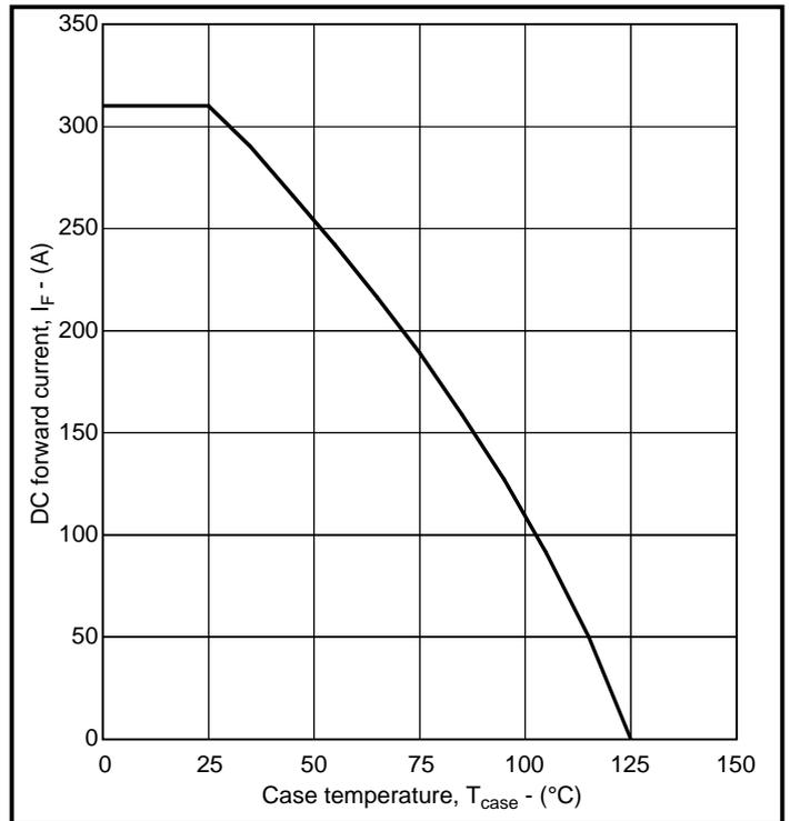
Fig. 6 DC current rating vs case temperature
