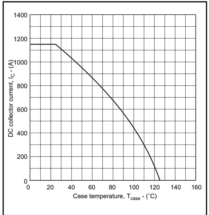
Fig. 12 DC current rating vs case temperature
