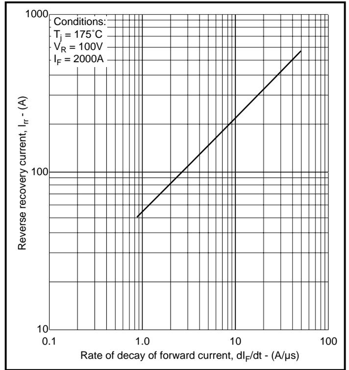
**Fig.5 Maximum reverse recovery current**
