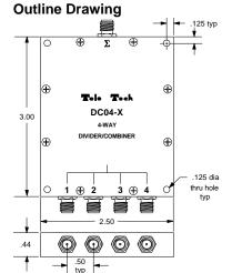
Matl Passivated Aluminum Connectors SMA (female) Stainless Steel
