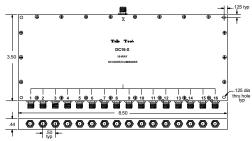
Matl Passivated Aluminum Connectors SMA (female) Stainless Steel
