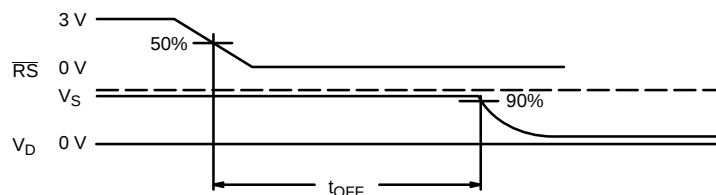
FIGURE 3. t_{OFF} from \overline{RS}
