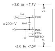
Measuring a single ended input voltage referenced to supply, i.e. the input voltage and the meter's power supply share the same 0V rail. Ensure solder link LREF is closed.
