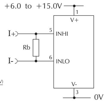
Measuring a current from a circuit which is floating with respect to the DPM's supply, i.e. the current and the meter's power supply are isolated from each other. Ensure solder link LCOM is closed.
