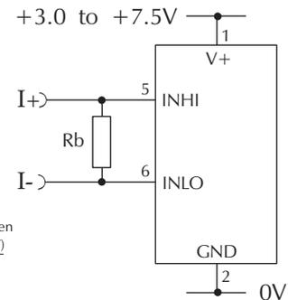
Measuring a current from a circuit which is floating with respect to the DPM's supply, i.e. the current and the meter's power supply are isolated from each other. Ensure solder link LCOM is closed.
