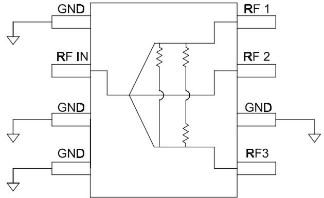
Pins labeled as ground should be DC and RF grounded.
