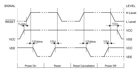
Please maintain the above sequence when turning on and off the power supply of the module. If  $V_{EE}$  is supplied to the module while internal alternate signal for LCD driving (M) is unstable or RESET is active, DC component will be supplied to the LCD panel. This may cause damage to the LCD module.
