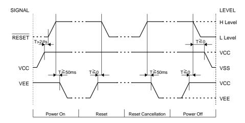
Please maintain the above sequence when turning on and off the power supply of the module. If  $V_{EE}$  is supplied to the module while internal alternate signal for LCD driving (M) is unstable or RESET is active, DC component will be supplied to the LCD panel. This may cause damage to the LCD module.
