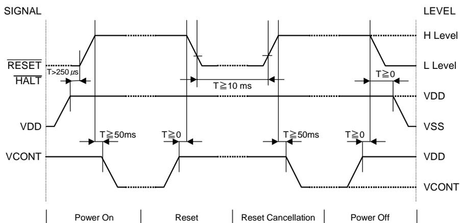
Please maintain the above sequence when turning on and off the power supply of the module. If  $V_{EE}$  and/or  $V_{CONT}$  is supplied to the module while internal alternate signal for LCD driving (M) is unstable or  $\overline{\text{RESET}}$  and  $\overline{\text{HALT}}$  is active, DC component will be supplied to the LCD panel. This may cause damage to the LCD module.
