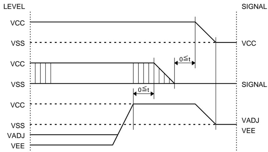
Please maintain the above sequence when turning on and off the power supply of the module. If  $V_{EE}$  and/or  $V_{ADJ}$  is supplied to the module while internal alternate signal for LCD driving (M) is unstable, DC component will be supplied to the LCD panel. This may cause damage the LCD module.
