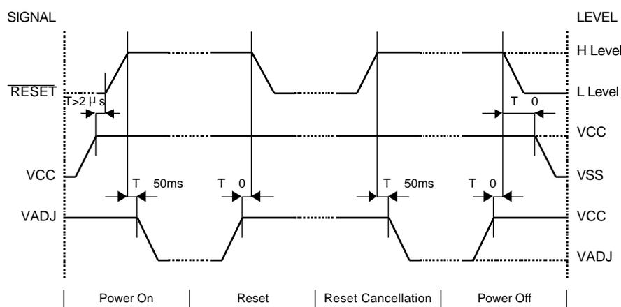
Please maintain the above sequence when turning on and off the power supply of the module. If  $V_{EE}$  and/or  $V_{ADJ}$  is supplied to the module while internal alternate signal for LCD driving (M) is unstable or RESET is active, DC component will be supplied to the LCD panel. This may cause damage to the LCD module.
