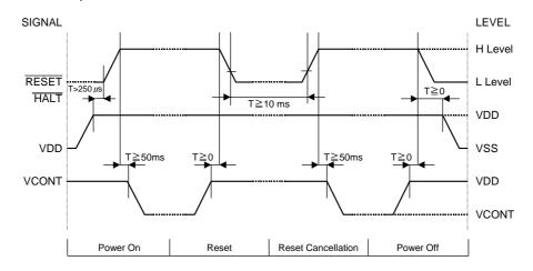
Please maintain the above sequence when turning on and off the power supply of the module. If  $V_{EE}$  and/or  $V_{CONT}$  is supplied to the module while internal alternate signal for LCD driving (M) is unstable or  $\overline{RESET}$  and  $\overline{HALT}$  is active, DC component will be supplied to the LCD panel. This may cause damage to the LCD module.
