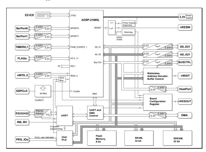
The D.Module family of DSP based Computer Modules offers a standardised hardware platform for embedded DSP applications. Mechanics and pinout are identical throughout the family members. 111 signals are reserved and provide identical functional-
