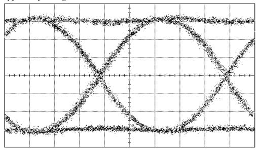
Input: 0 dBm p-p @ 10 GB/s, 1550 nm & 50% duty cycle
