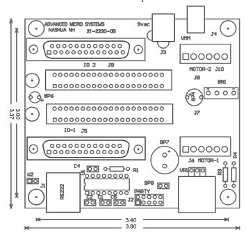
An RS-232 input converts standard serial voltages to TTL levels to drive up to 10 axis using Advanced Micro System's "Party Line" protocol. The open drain TXD outputs from each axis are wire-or'd, providing a party line communication method. Prior to operation each axis must be assigned a one character name that is stored in the DCB-26 NV memory. Removing the "Party Line" jumper and inserting one axis at a time facilitates name assignment.
