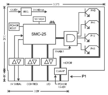
The 2 amp model (DCB-25-2) implements power Darlington transistors and a heat sink that widens the overall length of the board by .75 inches.
