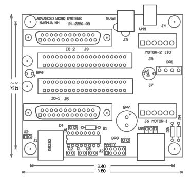
An RS-232 input converts standard serial voltages to TTL levels to drive up to 10 axis using Advanced Micro System's party line protocol. The open drain TXD outputs from each axis are wire-or'd, providing a party line communication method. Prior to operation each axis must be assigned a one character name that is stored in the DCB-25 NV memory. Removing the "party" jumper and inserting one axis at a time facilitates name assignment.
