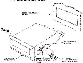
The low profile case is retained in a front panel cutout by sliding the DPM housing in through the cutout opening and securing the housing from the rear using 2 "L" brackets and screws. Proceed as follows:
