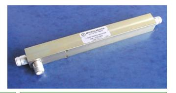
Microlab/FXR Model D2-55FN Two Way Power Splitter with N connectors, has been designed to evenly split high power cellular signals with DC continuity and minimal reflections or loss. All joints are moisture sealed to meet the IP65 rating. The mechanical shape allows simple attachment to pole or wall using the bracket provided.
