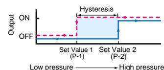
Note: The above figure is for the case when the output operation is set to NO (normally open).
