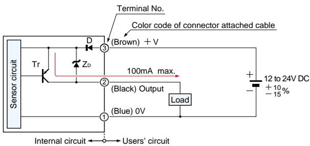
Symbols ... D : Reverse supply polarity protection diode
