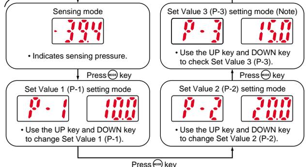
Note: Set Value 3 is only displayed when automatic sensitivity setting mode has been set. Furthermore, if Set Value 3 is between Set Value 1 and Set Value 2, the UP key and DOWN key can be used to correct it.
