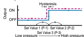
Note: The above figure is for the case when the output operation is set to NO (normally open).
