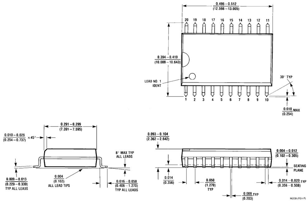
**20-Lead Small Outline Integrated Circuit (SOIC), JEDEC MS-013, 0.300 Wide
