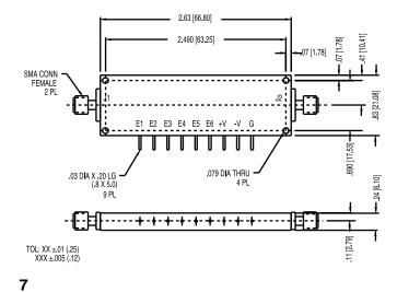
Dimensions in parentheses are in millimeters and for reference only.
