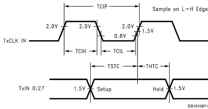
FIGURE 5. DS90CR287 (Transmitter) Setup/Hold and High/Low Times
