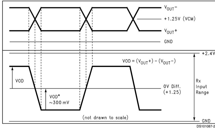
FIGURE 19. Single-Ended and Differential Waveforms
