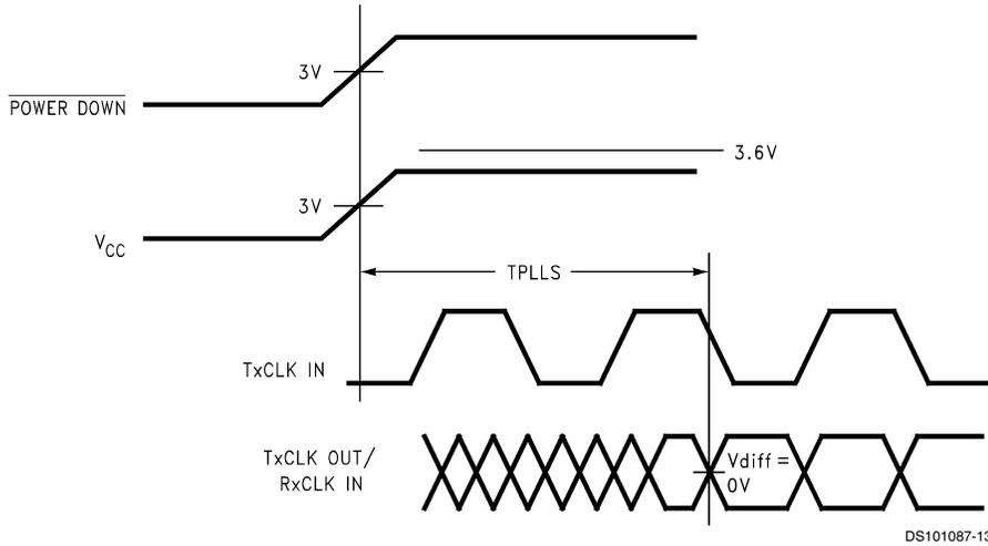
FIGURE 9. DS90CR287 (Transmitter) Phase Lock Loop Set Time
