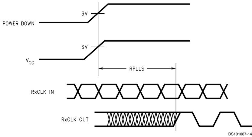
FIGURE 10. DS90CR288A (Receiver) Phase Lock Loop Set Time
