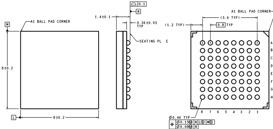
DIMENSIONS ARE IN MILLIMETERS
