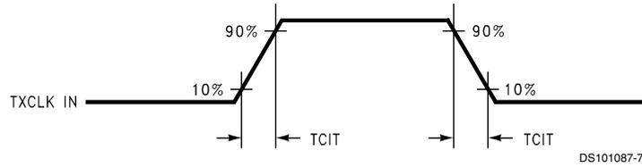
FIGURE 4. DS90CR287 (Transmitter) Input Clock Transition Time
