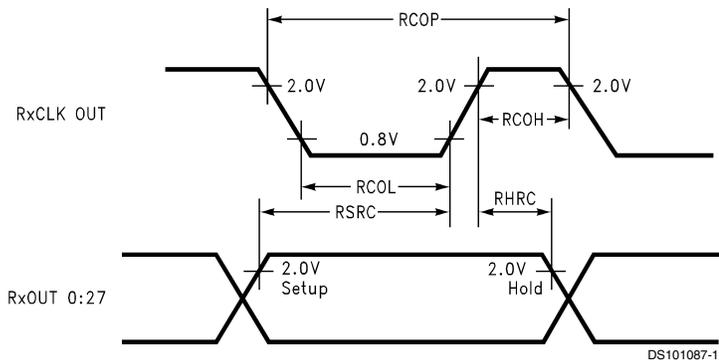
FIGURE 6. DS90CR288A (Receiver) Setup/Hold and High/Low Times
