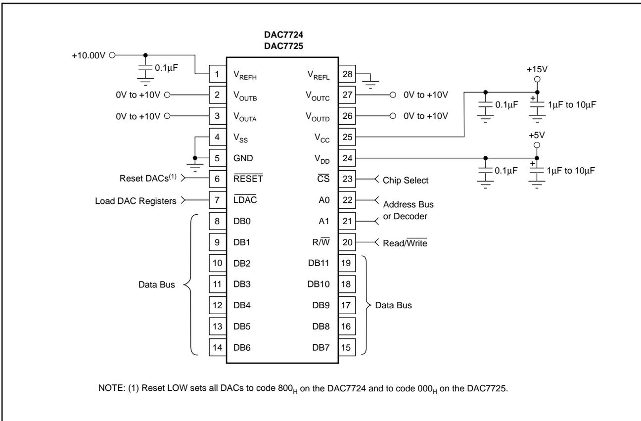
FIGURE 2. Basic Single-Supply Operation of the DAC7724/25.
