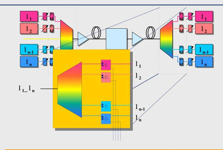
P. Neumann FO ON 17.9.2001 Page 4 Integrated optical de-coupling and opto-electrical conversion
