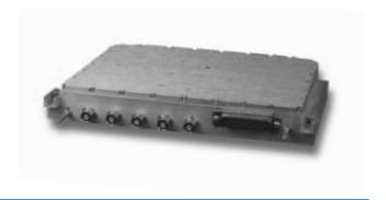
This high speed indirect synthesizer contains two parallel, indirect synthesizers, and offers fast hopping between channels. Under the control of the input tune word, each dual phase lock loop synthesizer is tuned to within 5 degrees of phase settling in 25 microseconds while additional logic allows for channel to channel speeds of 500 nanoseconds maximum.
