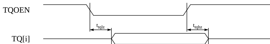
FIGURE 5. Synchronous Single-Port SRAM Test-Data Output-Enable Timing
