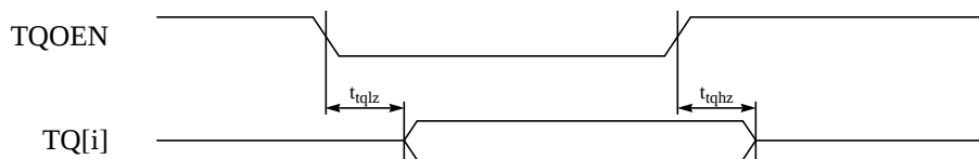
FIGURE 11. Synchronous Single-Port SRAM Test-Data Output-Enable Timing
