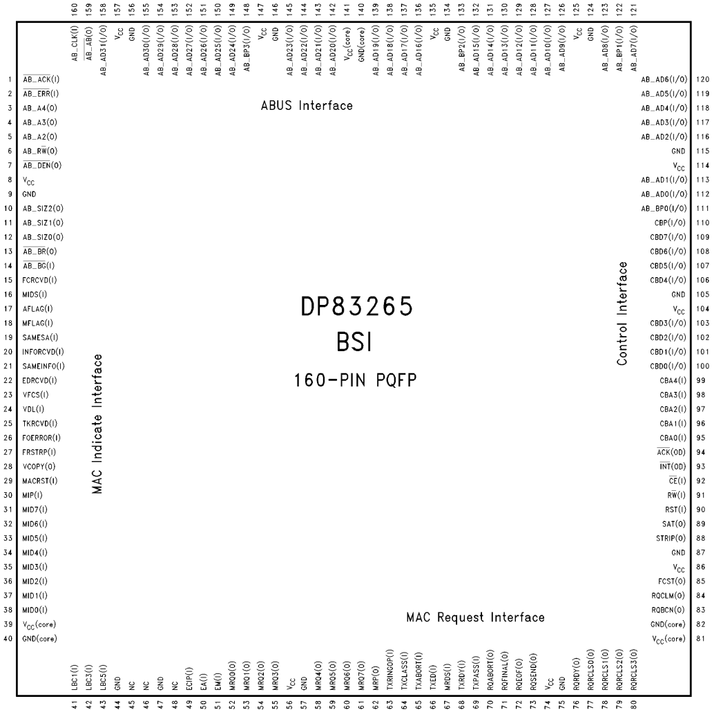
FIGURE 6-1. DP83265 160-Pin Pinout
