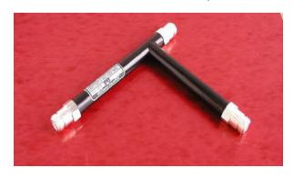
Microlab/FXR DH series Unequal Power Splitters unevenly split high power cellular signals with minimal reflections or loss over the cellular, PCS and UMTS bands. Shown are models for the ratios of 90:10 and 97:3, equivalent to 10 and 15 dB taps. Similar models are available with split ratios from 6 to 20 dB.
