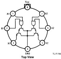
Pin 4 is in electrical contact with the case
