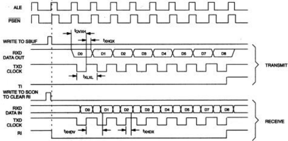
SERIAL PORT 0 (SYNCHRONOUS MODE)
