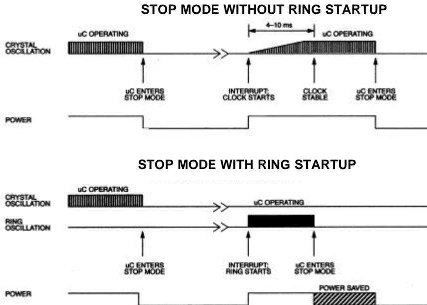
Note: Diagram assumes that the operation following Stop requires less than 18 ms to complete.
