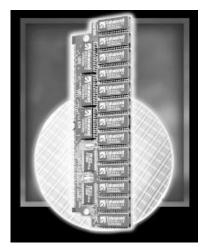
The DM4M32SJ achieves 4Mb x 32 density by mounting 32 4M x 1 EDRAMs, packaged in 28-pin plastic SOJ packages on both sides of the multilayer substrate. Four buffers have been added to reduce the loading on the address and control lines. The buffers have balanced output current levels and current limiting resistors. These offer low ground bounce, minimal undershoot, and controlled fall times.
